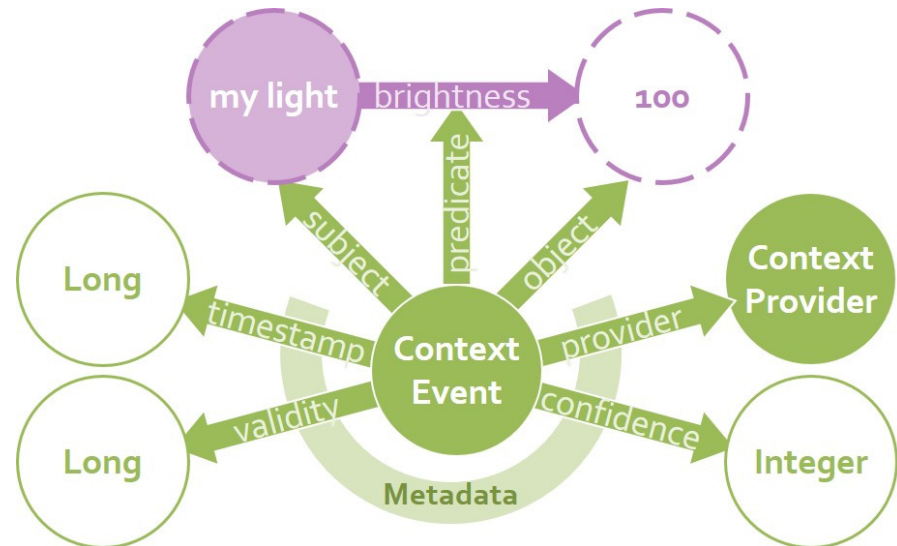
A Context Event is composed of the mandatory SpO triple and some metadata
